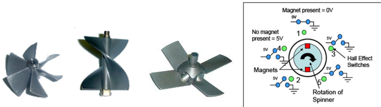
Fig. 17.C.2 – Various types of spinners – Schematic of the Hall effect – Courtesy Sondex
