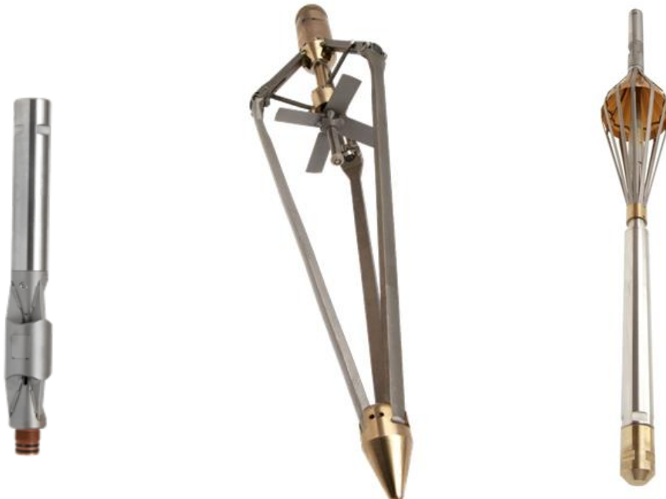
Fig. 17.C.3 – Inline, Fullbore and Petal Basket flowmeters – Courtesy Sondex
