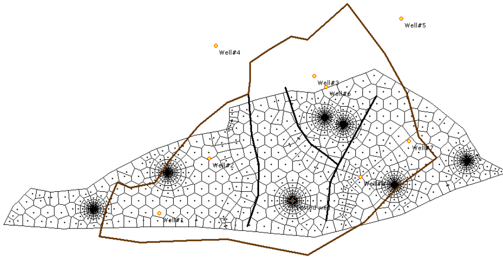
Fig. 14.E.9 – Equivalent Voronoi grid for an anisotropic reservoir ( k_x/k_y=0.2 )
