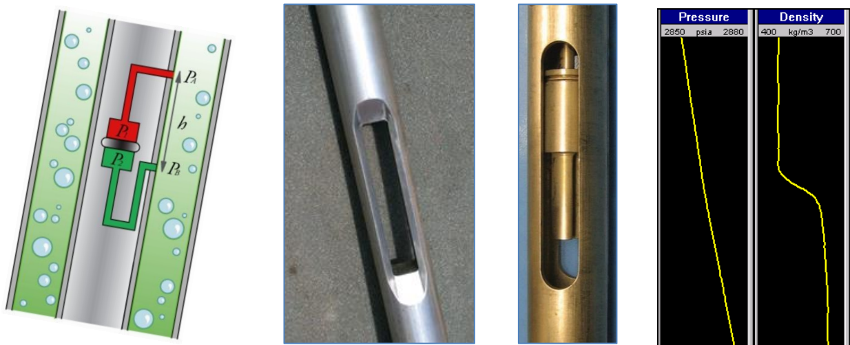
Fig. 17.C.5 – Schematic of a gradiomanometer; nuclear density tool; TFD tool; pressure differentiation
